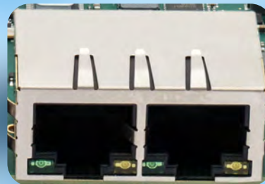
Dual 2.5 Gigabit Ethernet
