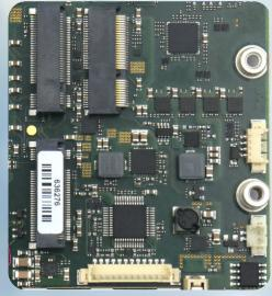
Triple M.2 Sockets / WLAN\_BT / 4G\_5G
